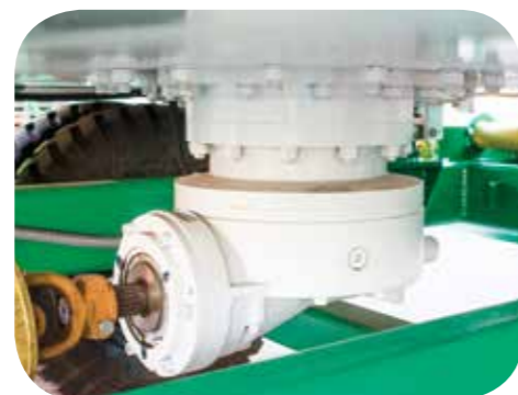
Transmission by gear reducer
