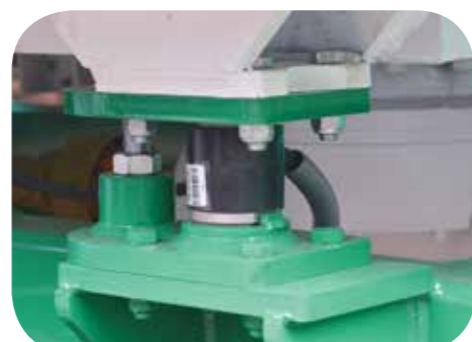
Load cells with reinforced supports
