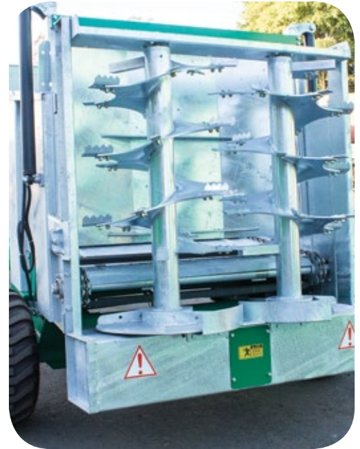
New high capacity spreader system with galvanized steel augers.
