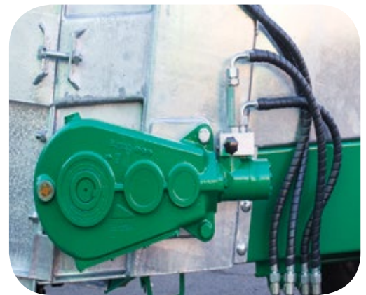
Hydraulic motors: allows higher accuracy in the distribution control and longer lifespan.
