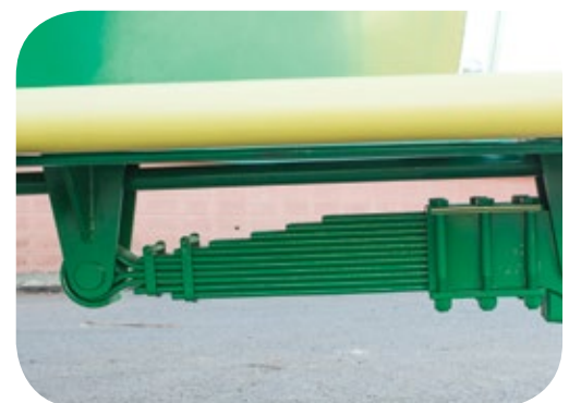
Exclusive head with leaf spring suspension system.
