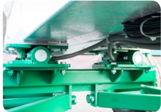
Robust load cell system and brackets for field operation.
