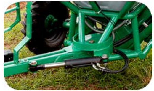
Shaft with lateral displacement during discharge (up to 1m).
